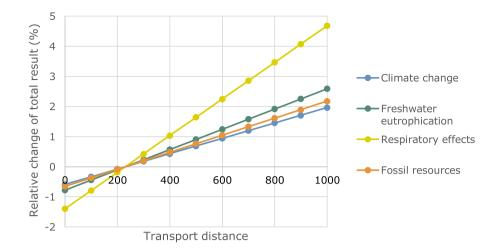
Fig. 7. Sensitivity analysis for transport distance (averaged for all variants).
