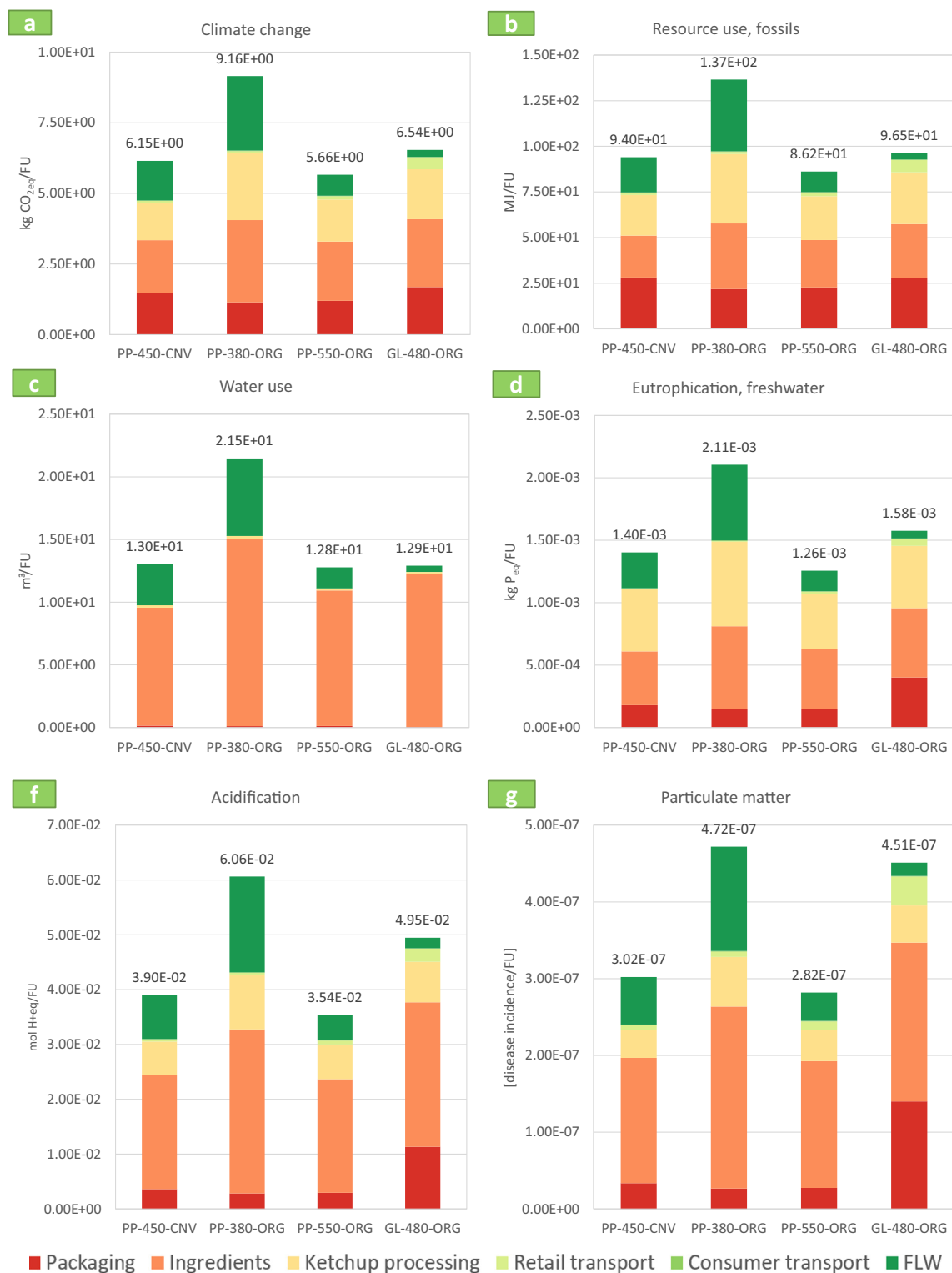
Fig. 3. Life cycle assessment results of most relevant impact categories for ketchup. Abbreviations for products represent (i) the packaging material as polypropylene (PP) or glass (GL), (ii) the content of bottles of 380, 450, 480 or 550 g and (iii) if the ketchup is a product of conventional (CNV) or organic (ORG) agriculture.
