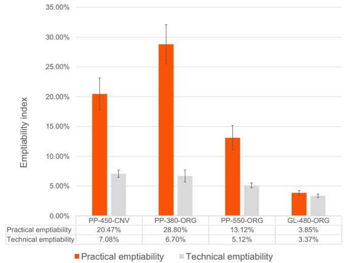
Fig. 2. Emptiability results of examined ketchup products. Bars represent the mean, while error bars are 95% confidence intervals ( $n = 6$ ). Abbreviations for products represent (i) the packaging material as polypropylene (PP) or glass (GL), (ii) the content of bottles of 380, 450 or 550 g and (iii) if the ketchup is a product of conventional (CNV) or organic (ORG) agriculture.
